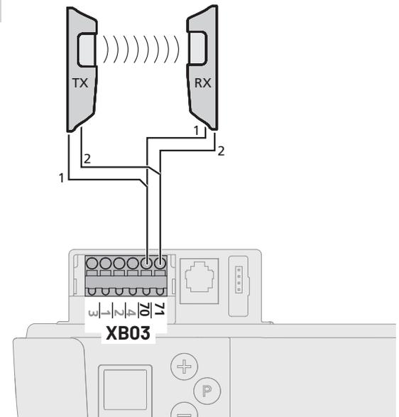
A connected photocell is automatically detected by the controller as soon as the power supply is connected. The photocell can be retrospectively reprogrammed. Unwanted photocells must be disconnected before the power supply is connected, otherwise the controller will detect them.
